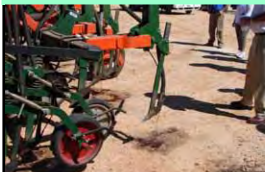
The planting tyne on Brosnans planter, with liquid injection tube at the back of the boot .
