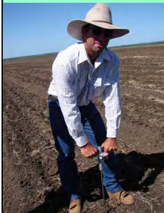
David Comiskey, "Melton" Alpha testing the penetrometer—measure soil strength.
